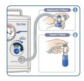
Adjust max pressure control knob clockwise or counterclockwise to set desired max pressure.
